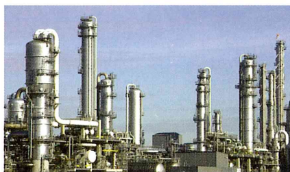
Petroleum undergoes fractional distillation in an oil refinery.
